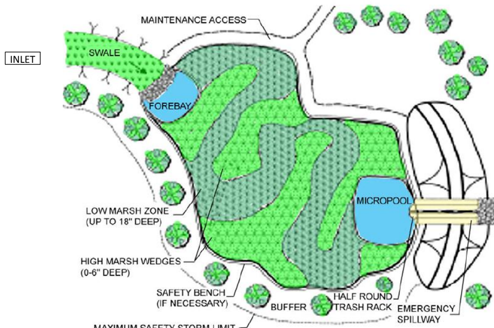
FIGURE 2: TOP VIEW OF POCKET WETLAND LAYOUT ADAPTED FROM BMP (BMP: CONSTRUCTED WETLAND 4)
